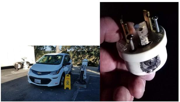
The Hampton Inn at Red Bluff was happy to 'cone' a charging station for us. However, after charging for a while I checked and the wires felt hot. (Always good to check the cables during a charge for excessive heat.) The very hospitable staff loaned me a screwdriver to wire my NEMA 14-50 plug directly into the charging station. Michelle helped by bringing me a headlamp when it started getting dark. All went well and we enjoyed this Inn's pool & views.
